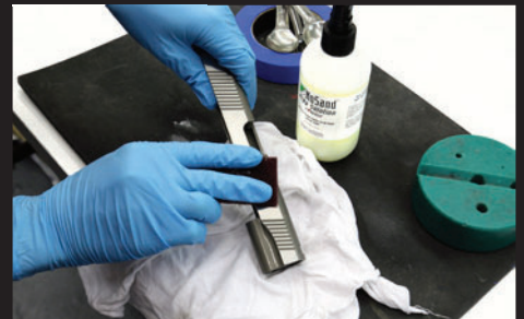
3rd. Use included scrubbing pad to work NoSand™ Prep Solution into all areas
