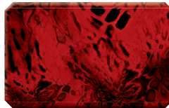
Red #74RD 4 oz Matte Black, 2 oz Gray Wolf, 2 oz Primary Red, 1 oz Hardener
